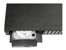
4 - Push the hard drive drawer back into the DVR and lock the drawer
